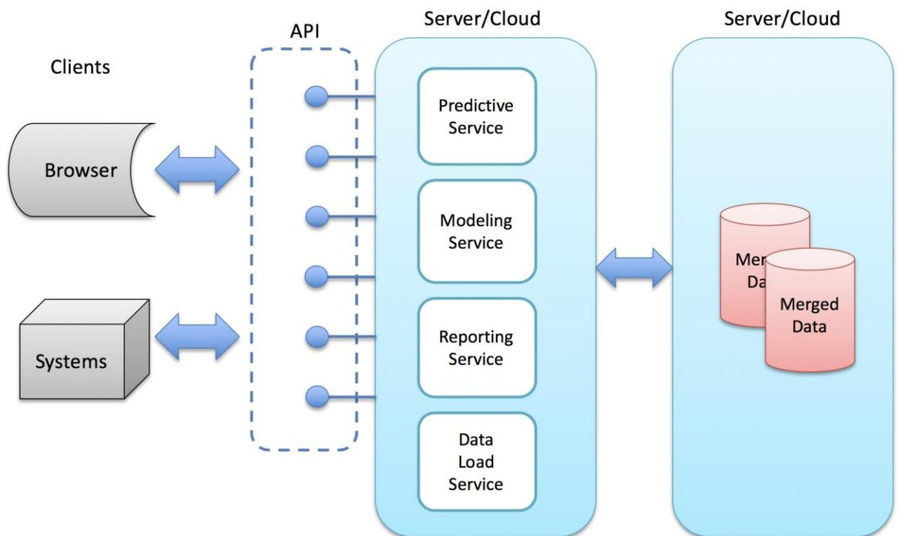
Note that the system provides a logical API layer, through which a variety of system integration and human interface functionality is managed.
